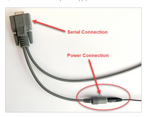
b) Connect the serial connector to the blue serial- to-USB (RS232) adapter.
